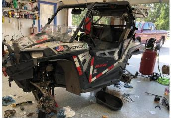
We also put in a brand new fuel pump to replace the bad one and tore into the engine as well. We did a compression test and one was WAY low, around 90 psi, the other was about 130 psi. We were hoping it was just the valves needing adjustment, and long story short, it was.
